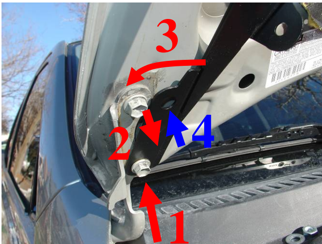
Hood-side bracket mounting
